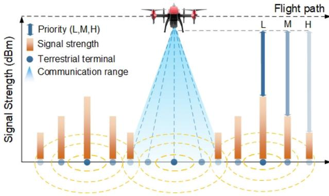
Fig. 8. Signal strength-based priority strategy for data transmission.
