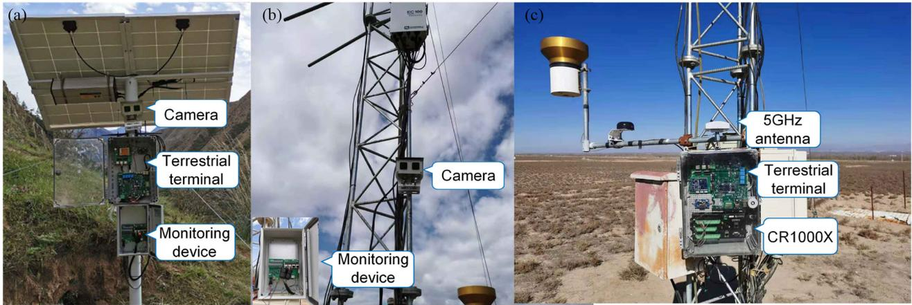
Fig. 10. Developed terrestrial terminals deployed for phenology and environmental monitoring. (a) Terrestrial terminal integrated with a wireless transceiver and phenology camera deployed to monitor Qinghai spruce (*P. crassifolia*) (N38.34°, E 100.17°, 2690 m a.s.l.) and arid desert meadow (N38.77°, E 100.32°, 1829 m a.s.l.). (b) Terrestrial terminal integrated with a wireless transceiver and CR1000X datalogger deployed to monitor the soil temperature (N 38.77°, E 100.32°, 1829 m a.s.l.).
