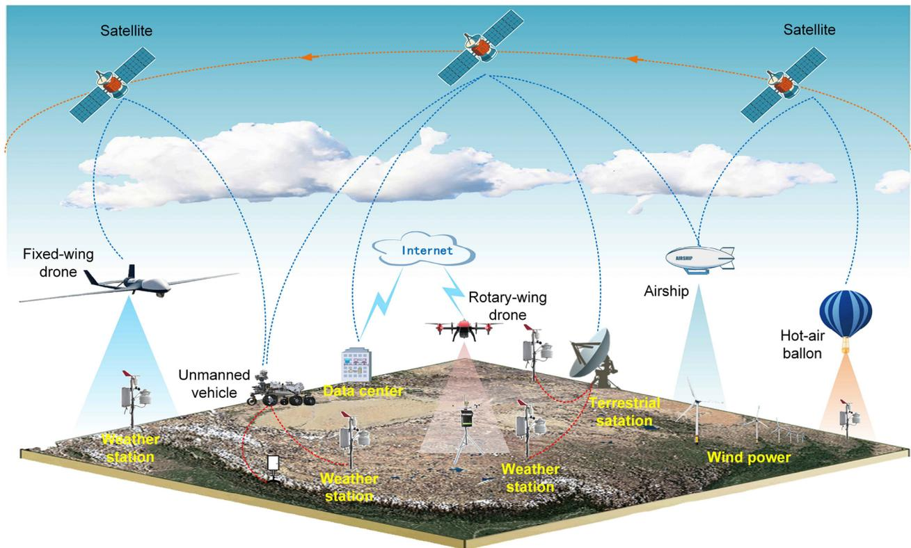
Fig. 1. Framework of the driverless-based IoRT network for ecosystem monitoring in extreme farmost environments.
