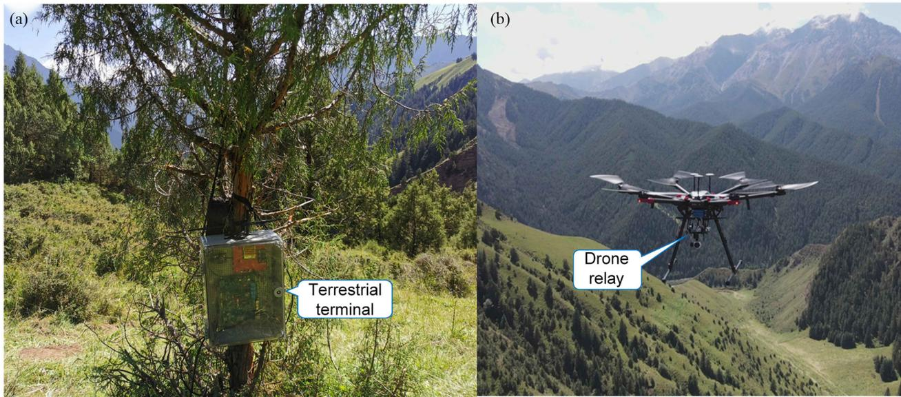
Fig. 4. Hardware system of the drone-enabled IoRT network, including (a) terrestrial terminal and (b) drone relay.
