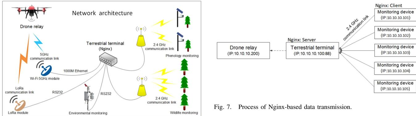
Fig. 6. Framework of the drone-enabled IoRT network.
