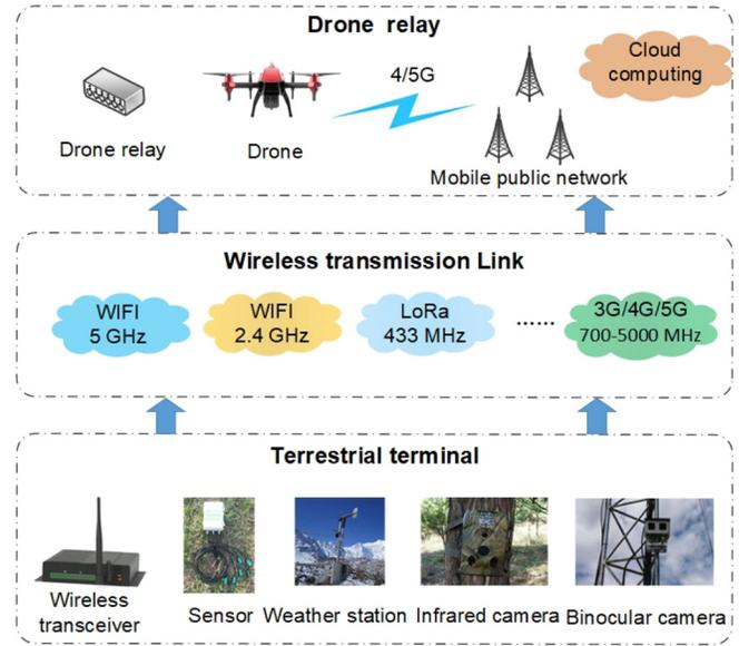
Fig. 2. Network architecture of the drone-enabled IoRT.
