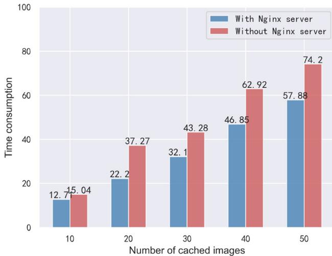
Fig. 15. Performance comparison of the system with and without Nginx server.
